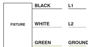
**NOTE:** POLE MUST BE PROPERLY GROUNDED. TO ENSURE PROTECTION, THE EARTH GROUND WIRE (GREEN) MUST ALSO BE CONNECTED TO THE POLE GROUND LUG. FAILURE TO DO SO CAN REDUCE OR ELIMINATE SURGE PROTECTION, RESULTING IN POSSIBLE DAMAGE TO THE LUMINAIRE.
