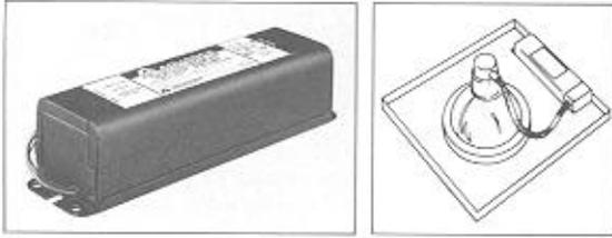
Also designed for indoor applications, these ballasts are encased and potted in Fluorescent ballast type cans and utilize Class A (90°C max.) insulating materials (the same as used in fluorescent lamp ballasts) for normal indoor ambients. This insulation is primarily used to minimize inherent ballast noise.
