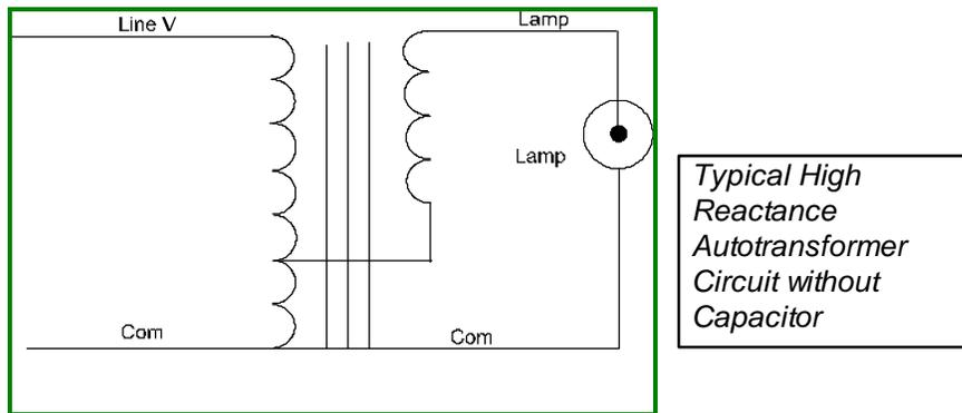
When the input voltage does not meet the starting voltage requirements of the HID lamp, such as 120, 208, or 480 volts for Mercury Vapor, a high reactance autotransformer ballast can be used to ballast the lamp. This will provide operating characteristics equal to the reactor.
