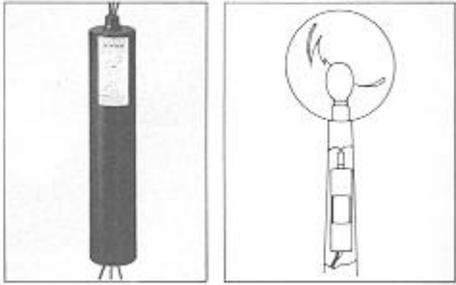
Lantern type fixtures mounted on slender poles require ballasts, which fit into the poles. Special, elongated core & coils are encased and potted in high temperature resin (Class H, 180°C max.) in cylindrical cans having a 2 9/16" outside diameter so they can be placed within all poles having a greater inside diameter. All include the leads necessary for direct connection to a photocell.
