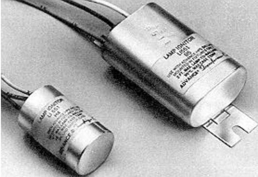
In order to start the lamp, an electronic component called an ignitor must be included in the circuitry of all High Pressure Sodium and certain new low-wattage Metal Halide lighting systems. This ignitor provides a pulse of at least 2500 volts peak in order to initiate the lamp arc.
