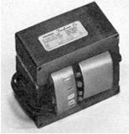
Quadri-Volt ballasts are also ideal for applications where an incandescent lamp is incorporated in the fixture. This provides immediate standby lighting in the event power is momentarily lost, extinguishing the HID lamp, which then must go through its restrike phase. The 120 volt tap can be connected, via a relay, to power a 120-volt incandescent lamp until the HID lamp has cooled sufficiently to restrike.
