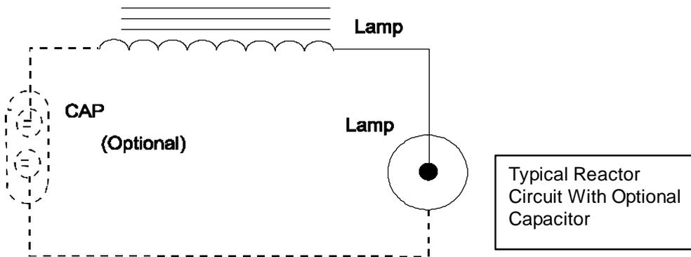
When the input voltage to a fixture meets the starting voltage of an HID lamp, a reactor ballast may be employed to operate the lamp. The necessary lamp starting voltage comes from the input voltage to the ballast. Because most Mercury lamps are designed to start at 240 or 277 volts, the reactor ballast is the most economical way to ballast a Mercury lamp in systems operated at either of these two input voltages.
