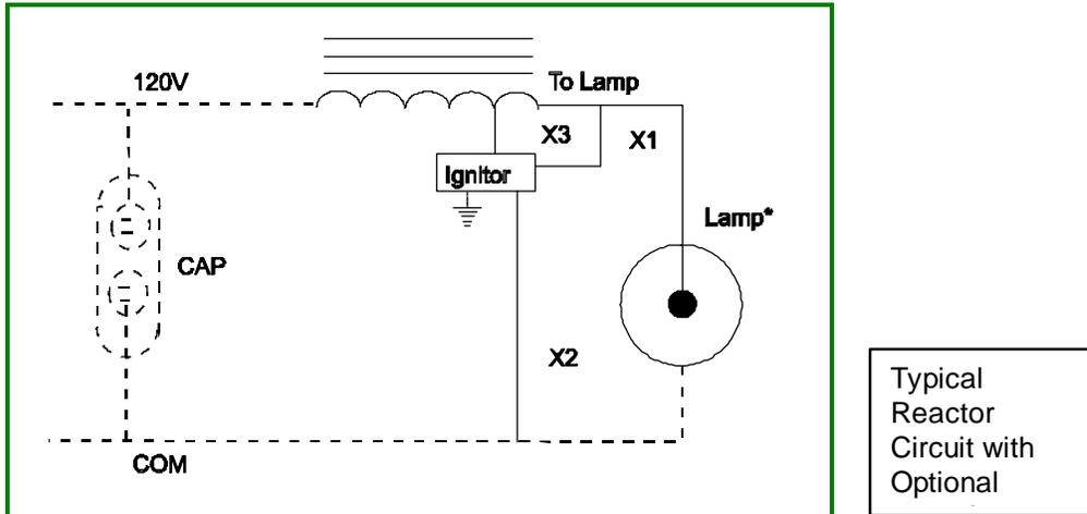
For an input of 120 volts, the simplest and most economical way to ballast a 35 thru 150 watt (55-volt) lamp is by utilizing reactor circuitry because these lamps require a 120 volt open circuit starting potential. Here, the reactor performs only the basic function of controlling current through the lamp.
