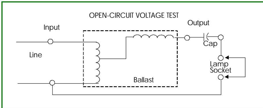
As an alternative, this test may also be performed simply by screwing an adapter into the lamp socket for easy access. Then hook up the voltmeter to this adapter. Reading must be within test limits shown.
