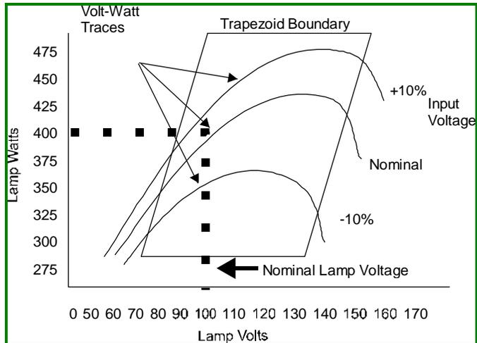
Taken from an Advance data sheet describing the 77A8402 series ballast operating a 400 watt HPS lamp, this volt-watt trace includes curves at nominal input voltage, at plus 10%, and at minus 10% of nominal. The portions of the curves within the trapezoid boundary define operation for this particular lamp-ballast combination over the life of the lamp.
