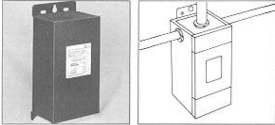
These units are designed for use indoors where the ballast must be mounted remotely from the luminaire. They are most typically used in factories where the luminaire may be mounted in a high bay where high ambient temperatures may be experienced. In these instances the remotely mounted ballast operates cooler, providing subsequent longer life.
