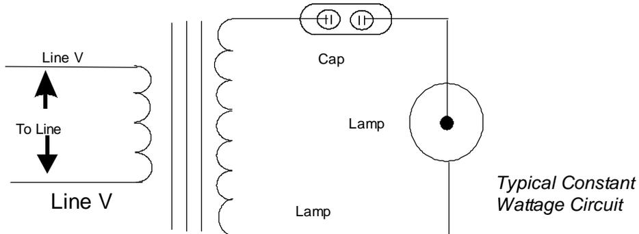
Sometimes referred to as premium constant wattage, this type of ballast will provide the highest lamp regulation available. Because there is no connection between the primary and secondary coils, this isolated circuit provides a safety factor against the danger of shock hazard.
