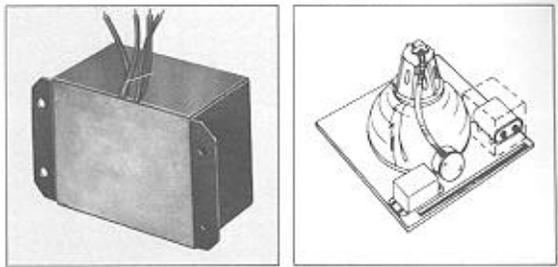
For indoor applications of HID lighting fixtures, such as in offices, schools and retail stores, ballast noise must be minimized. For these uses, standard ADVANCE core & coil ballasts are encased and potted in a high-temperature resin (Class H, 180°C max.) and secured to the fixture through integral mounting flanges on the ends of the case. As with the basic core & coil, the capacitor (and ignitor of HPS lighting) must also be mounted separately in the fixture.
