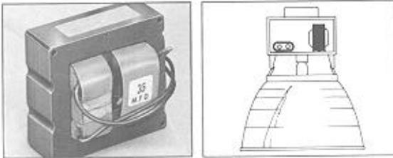
The most basic of all shapes is the core & coil which may also be used by itself as a component of a fixture, but is also used to form the nucleus to the five other ballast configurations detailed in this section. It consists of one, two or three copper coils on a core (or "stack") of electrical grade steel laminations. As shown here, the core & coil ballast will be mounted within a fixture housing by the luminaire manufacturer. It represents today's most popular method of utilizing a ballast.
