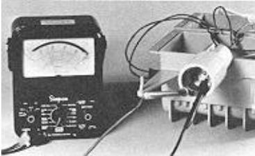
Open Circuit Voltage rest at Socket
