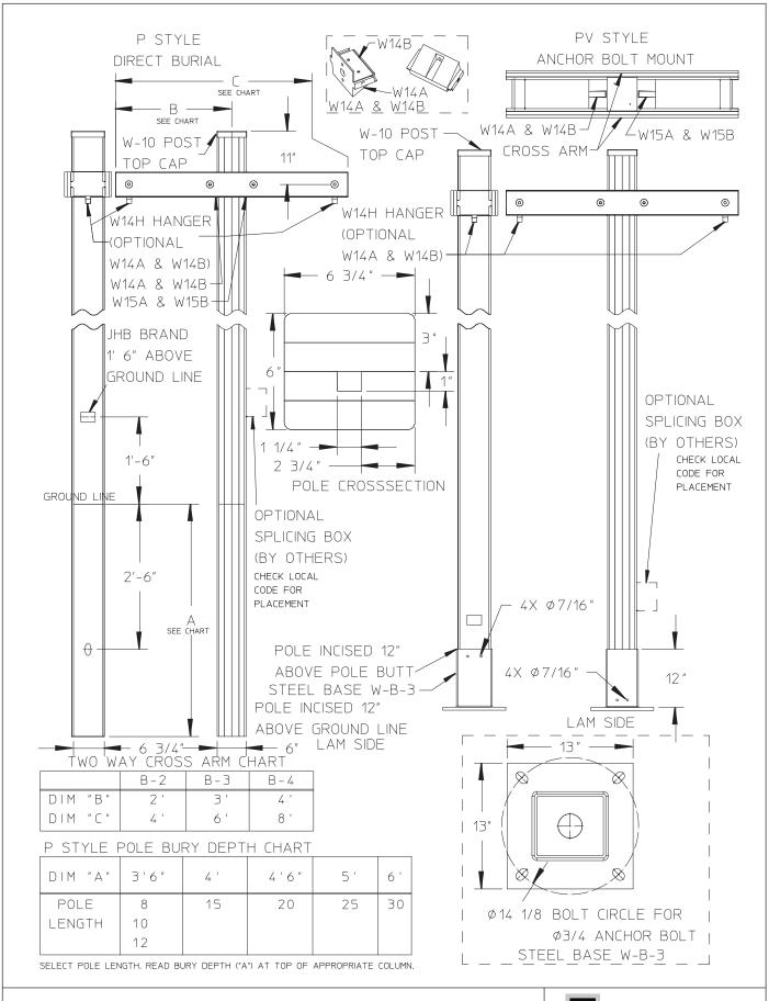
6-3/4" X 6" P AND PV SIDE MOUNT STRAIGHT POLE SPECIFICATION WITH TWO WAY CROSS ARM
